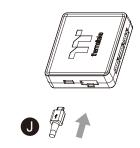
If you want to connect two or more connectors, you can use the bridge cable to connect the controllers.
